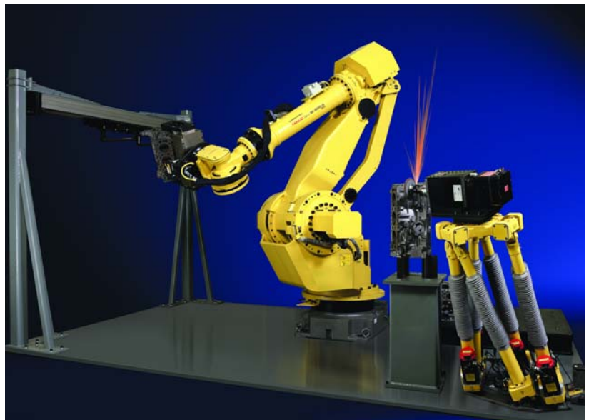
Engine block handling and deflashing with Intelligent M-900iA/350kg and F-200iB robots.
